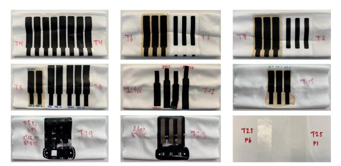
Figure 10: Pictures of samples used in wash durability testing. Pictures taken after 15 wash cycles.
