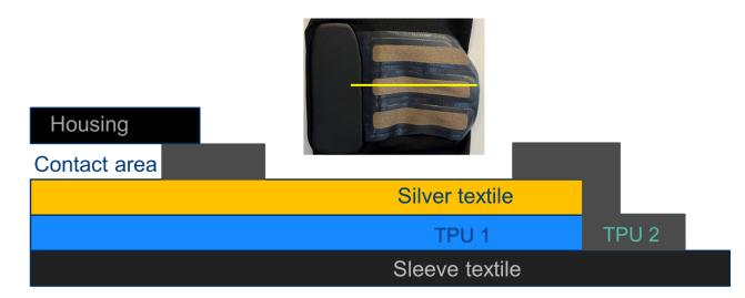
Figure 1: Picture of the EMG electrode part of MLI ELBOW, and a scematic of the design along a line indicated on the picture. TPU (Thermoplastic PolyUrethane) is a highly stretchable polymer.
