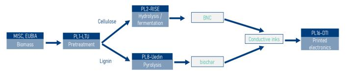
Figure 4: Process flow for the production and use of BNC and biochar
