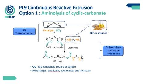
Figure 5: First approach evaluated to synthezise biobased NIPUs: step-growth polyaddition of cyclic dicarbonates and diamines.
