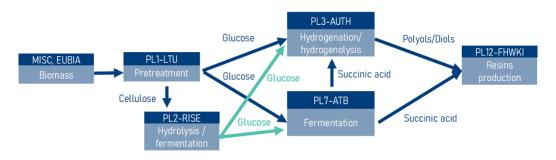
Figure 2: Process flow for the diols and succinic acid used by PL12 in the production of PUDs.
